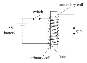
The switch is closed and the current in the primary coil increases to a maximum value. The switch is then opened and the current falls to zero almost immediately. The secondary coil produces a large p.d., creating an electric field strong enough to cause a spark across the gap.
